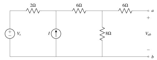
i. (4 points) Find the Thevenin equivalent resistance between terminals *a* and *b*.
