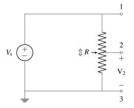
In the figure, the potentiometer is connected to a voltage source. Express the output voltage,  $V_2$  (the voltage at terminal 2), as a function of the source voltage  $V_s$ ,  $R_{12}$ , and  $R_{23}$ .
