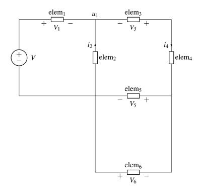
(b) (1 point) Using your labeled voltages/currents, write the KCL equation for node  $u_1$ .
