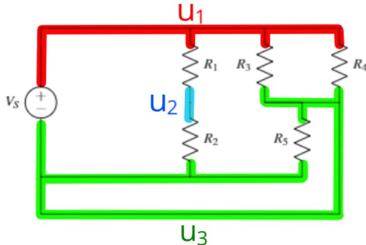
represent the same circuit behavior. This is useful because sometimes it is easier to see patterns in a circuit diagram if it's drawn differently. However, we must be careful to not change the circuit when we redraw it.
