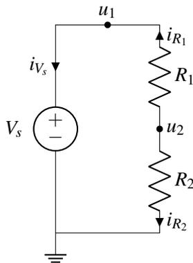
What are the  $+/-$  labels for  $R_1$  and  $R_2$  according to passive sign convention? (See Note 11B for explanation of passive sign convention)
