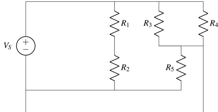
We'll find nodes one at a time with this method (the order we find the nodes is arbitrary). We start by choosing a color to represent the first node (red, in this example). Then we choose a starting point on the circuit, such as the upper left corner. From this point, we trace (in red) along all of the connected wires until we hit a non-wire component. Everything traced in red is part of a single node.
