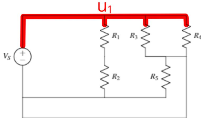
Then we choose a new color and a new point on the circuit *that is not already colored*. We repeat the process: tracing over all wires that are connected to this new point and stop when a non-wire element is reached. Repeat this process for new colors until all of the wires have been identified.
