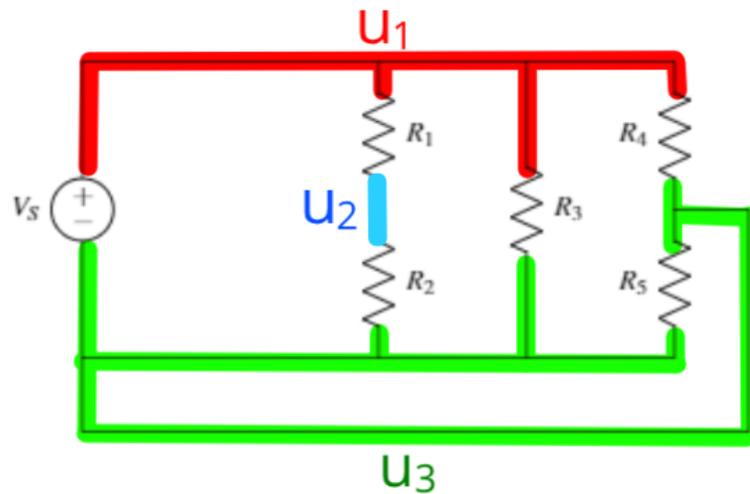
We can similarly rearrange other components if needed. In this case, we move  $R_5$  but maintain that it is connected to the green node,  $u_3$ , on both sides. Note that all of the elements have the same node connections as they did in the original circuit. Therefore this circuit will have the exact same behavior as the original:
